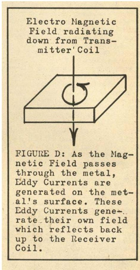
These currents, called “eddy currents”, generate their own electromagnetic field the same did the coil when it got its current from the oscillator. This “eddy current” field radiates out in all directions the same as did the coil’s field. A portion of the “eddy current” field is radiated upward and reaches the detector’s receiver coil where it is “picked up” or its presence is detected. See Photo 2.
